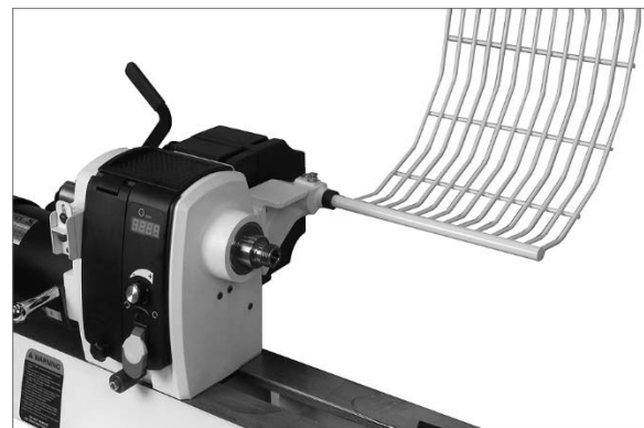
Figure 5-5: guard (optional) tilted back
