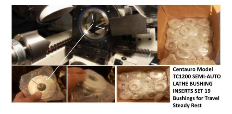
CENTAURO MODEL TC1200 19 peace bushing set inserts for traval steady rest ,size range : 1 1/8" dia to 3 15/16" in 1/8" increments.
